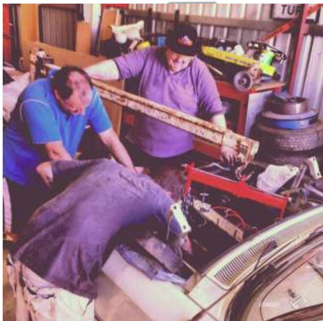
Once the old motor was out, parts were removed and found the main cause the engine no longer ran was the starter motor, it had given its last crank down to slices of carbon brush left to transfer the power to the now heavily oiled starter (could have been a hydraulic pump).
